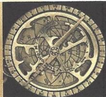
Figure 2. Astrolabe is an elaborate inclinometer capable of working out several kinds of problems in astronomy, first described by Khwarizmi.
